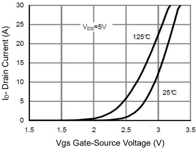
**Figure 2 Transfer Characteristics**
