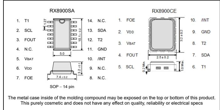
The metal case inside of the molding compound may be exposed on the top or bottom of this product. This purely cosmetic and does not have any effect on quality, reliability or electrical specs
