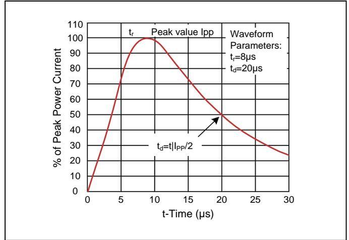
Figure 3. Non-Repetitive Peak Pulse vs. Pulse Time
