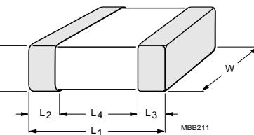
**Fig. 2** Surface mounted multilayer ceramic capacitor dimension
