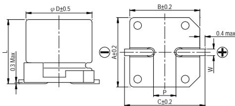
Lead Spacing and Diameter Unit: mm
